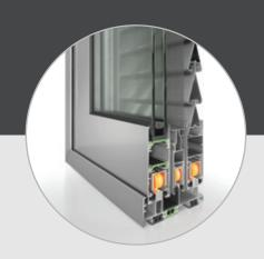
A basic sliding window system, with thermal break, capable to support a large variety of solutions. It is ideal for replacing older windows in existing buildings. It offers a wide range of cross-section options and multiple types of locking mechanisms and handles. It provides stainless steel rail and integrated flyscreen and/or shutter.
